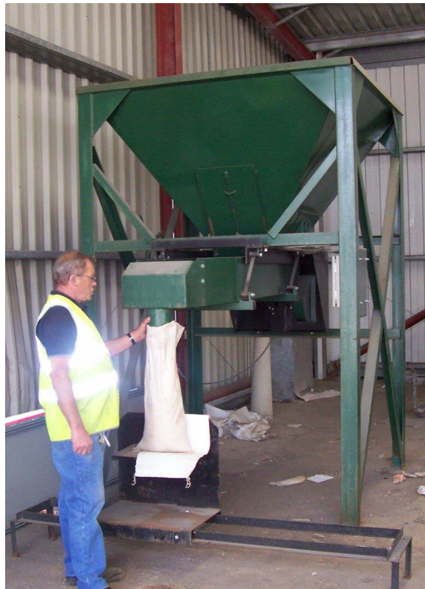
Rapid sandbag filling machine in use at a Council depot
